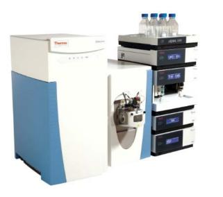
Capable of separating mass fragments at the fifth decimal place (exact mass) where MS/MS instrumentation was limited to single-digit mass unit
